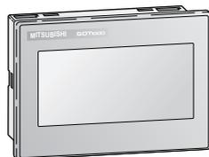
The new **GT1020** series has a bright 3.7-inch STN black-and-white liquid crystal display with 3-color backlight for use in a variety of display applications. Recipe management, alarming and messaging are included as standard. The unit has a built-in memory for up to 4000 16-bit data words which can be used to store or exchange data with a connected PLC. The GT1020-LBD/-LBL have a RS422 and a RS232 terminal and the GT1020-LBD2 has a RS232 terminal only.
